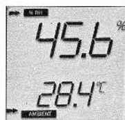
Figure 3: Typical Screen Display During Operation
