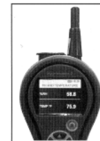
Figure 4: Hygromaster2 as a Hygrometer
