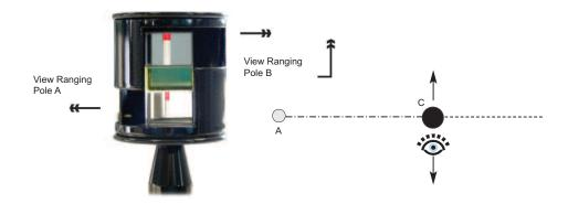
Take up a position roughly in line between Poles A and B. Look through the window and sight pole A in the lower window and pole B in the upper. Move forwards or backwards at right angles to the line until the two poles appear to coincide. The Optical Square is now in line between A & B and point C can be marked.
