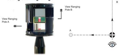
Hold the Optical Square over the alignment point, using either a plumb-bob or ranging pole to centre. Sight to Ranging Pole A through the lower prism. As Ranging Pole B is moved, view it through the centre window until the two images appear to coincide. The angle A to B is now 90° at the alignment point.
