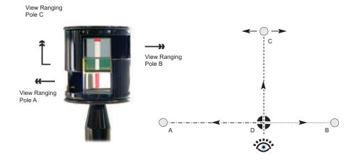
This is a combination of examples 1 and 2, as above. Start by setting the point on line between A and B, getting a coincidence in the prisms. Then move along the line towards Pole C, looking through the centre window. When the three poles line up, D is on line and ADC & BDC are at right angles.
