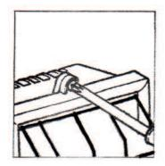
4. Carefully replace front surround, making sure it is correctly positioned. Screw up tightly.
