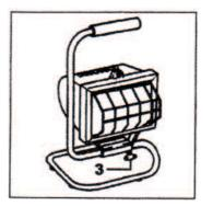
2. Lamp angle may be altered simply by loosening the angle adjustment knob (3) moving the stand handle to to bring the lamp to the desired angle, then tightening the angle fixing knob **Inserting or Replacing Halogen Lamp**
