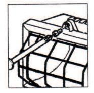
1. Unscrew retaining screw on top of lamp. This will release the protective grid, front surround and glass faceplate.
