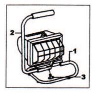
1. Insert stand base (1) into other end of tube. Use the stand handle (2) to position the lamp to the desired angle. Insert and tighten angle adjustment knob (3)
