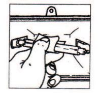
3. To insert halogen tube: unwrap globe, taking care your fingers do not touch the tube. Use wrapping to handle the tube. Push one end of tube into either of the spring-loaded sockets. Locate other end on other socket, and release.
