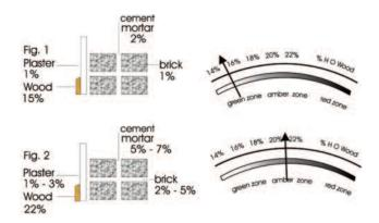
This diagram illustrates the different moisture contents of different building materials, all in moisture equilibrium. The upper example shows the air-dry (safe) condition; the lower example a wet (dangerous) condition. The figures on the right are WME readings on a Protimeter moisture meter.
