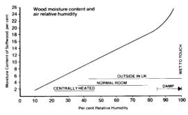
The graph shows the approximate relationship between the relative humidity (r.h) of air and the moisture content of typical softwoods. The horizontal lines show the typical range of humidities met in various circumstances. Wood kept in these environments will gradually come into equilibrium at the moisture content levels indicated on the vertical scale. 75% rh. is 'safe' in building materials.
